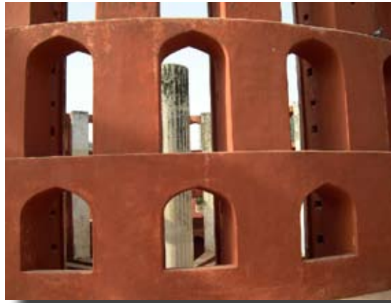
The Ram Yantra is a multifloor version of an Azimuth Instrument which also measures the altitude of heavenly bodies. At sunrise the shadow falls on the central pillar at what is essentially zero altitude.
