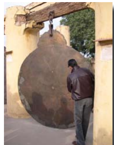
The Great Astrolabe is one of the largest astrolabes in the world. It is 3 meters tall and weighs 400 kg. It is a celestial map, engraved on a seven-alloy metal disk. The hole in the middle is the Pole Star.
